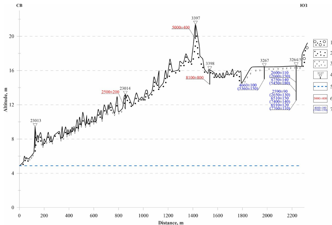
Fig. 1. Geomorphological profile of the Taipalovskii Bay shore. 1 – sand-gravel-pebble deposits; 2 – sands; 3 – peat; 4 – sampling points; 5 – water level on the day of leveling survey; 6 – OSL age; 7 – radiocarbon age, calibrated age is given in parentheses.
