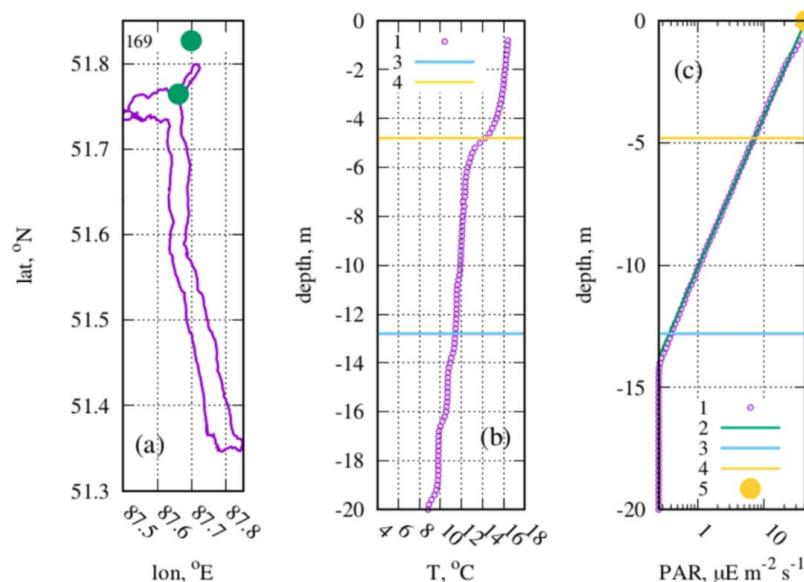
**Fig.2.** An example of simultaneous measurement of temperature profiles (b) and PAR (c) by the “CONDOR” instrument at station 169, carried out on August 17 in Kamga Bay (a), and the result of data processing: 1 – behavior of the profile of the measured parameter; 2 – linear approximation by equation (2); 3 – lower border of  $Z_{eu}$ ; 4 – lower limit of the UML; 5 – PAR(0<sup>-</sup>).
